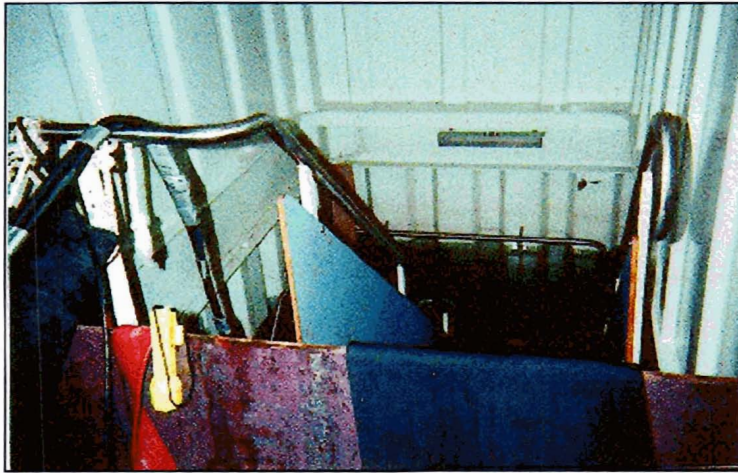
Deck 1, port side passageway. Note welded plate across stairwell put in place to limit the chance of progressive flooding.
